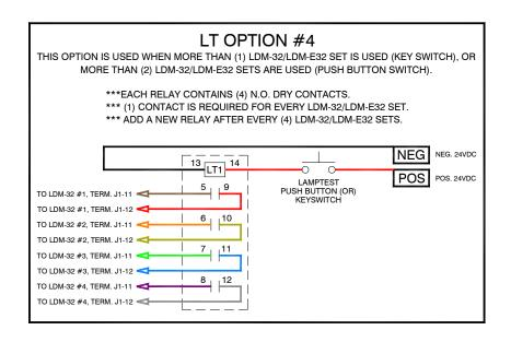
\*\*\*An LDM-32/LDM-E32 Set consists of (1) LDM-32 Driver and (1) LDM-E32 Expander Driver.
